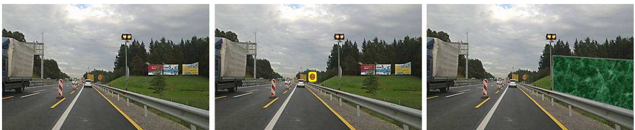
Figure 10 - Conspicuousness of traffic sign due to billboards (Enhance traffic sign and motorway screen as a contra measures)
