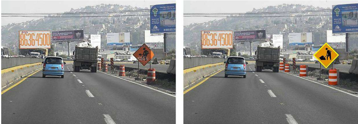
Figure 11 - Conspicuousness and clearness of traffic signage (On right picture is shown enhance traffic signage with proper quality and maintenance)
